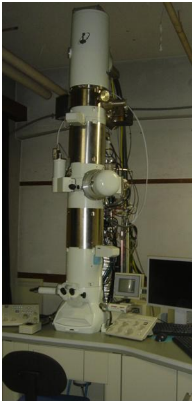
Aberration corrected TEM/STEM with 0.07 nm resolution
